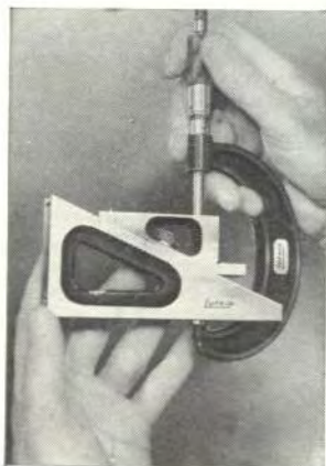
Gage Being Set to Micrometer Accuracy
